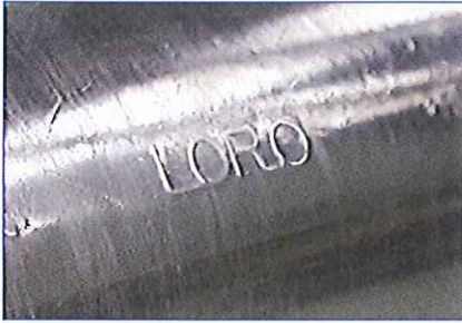
LORO-X pipes and fittings marking in longitudinal direction every 30cm.
