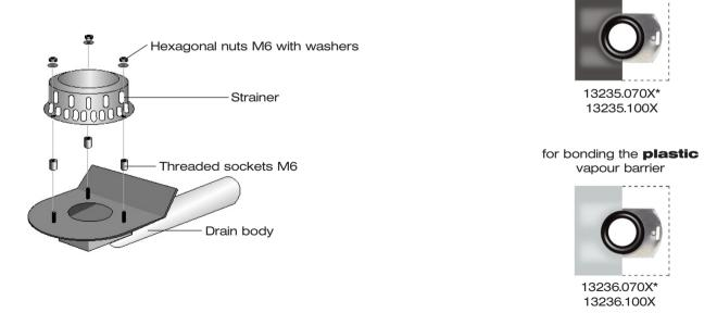
\* DN 70, incl. sealing element
