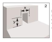
Make 10 mm diameter holes for the sliding flange with the factory-fitted connecting sleeve for connecting the vapour barrier according to the details specified in Table 2 (Fig. 2).
