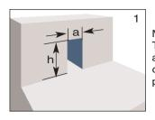
Make the parapet opening according to Table 1 (Figure 1). Make the hole as far as the bare slab so that the roof space can be drained during the construction phase.
