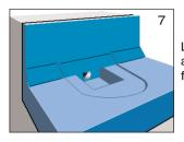
Lay the thermal insulation panels, and cut out sufficient space in the region of the drain to allow the drain to be fitted (Fig. 7). The fixed flange of the roof drain should, according to the flat roof regulations, be flush-mounted into the substrate.
