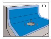
Apply bitumen primer to a width of 100 mm around the flange (observe the drying time). Cut the **connecting sheet** of the existing bituminous roof sealing sheet, with a size of 700 mm x 1000 mm, to size (Fig. 10), and join to the drain bonding flange in accordance with the laying instructions from the manufacturer of the roof sealing sheet.
