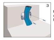
Fasten the sliding flange (with the connecting sleeve rolled up) using a screwdriver for slotted screws (Fig. 3).
