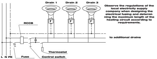
Heated roof drains can be connected individually or in parallel.
