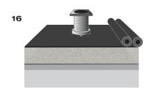
16 Clamp the drainage ring into the clamping ring of the drain body.
