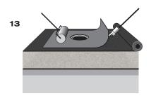
13 Remove the protection foil and unfold the connecting sleeve on the lower sealing sheet.
