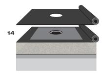
14 Roll out the <u>upper</u> sealing sheet over the drain. Prepunch the sealing sheet in the area of the drain.
