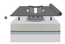
**8** Cut a circular hole into the sealing sheet in the area of the extension cartridge. Hole dimensions: DN 70 =  $\emptyset$  ca. 275 mm, DN 100 =  $\emptyset$  ca. 330 mm.
