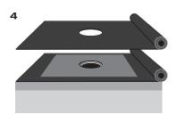
**4** Roll out the <u>upper</u> sealing sheet over the drain. Prepunch the sealing sheet in the area of the drain.
