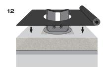
Prepunch the <u>lower</u> sealing sheet (in the case of a two-layer roof sealing). Hole dimensions: DN 70 =  $\emptyset$  ca. 275 mm, DN 100 =  $\emptyset$  ca. 330 mm.
