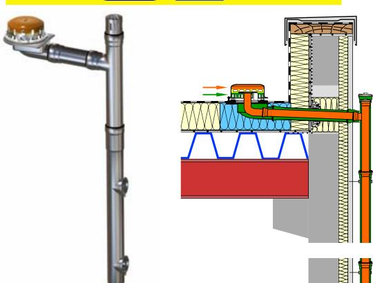
The LORO-X combined main & emergency system with the "pipe-in-pipe principle", for which LORO has applied a patent, unties a silent gravity main drainage with a silent power siphonic emergency drainage in a single drainage system.
