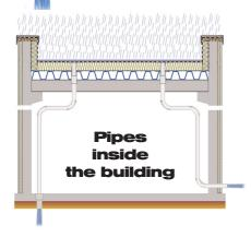
From pitched Roofs with Gutters and downpipe outside the building, it is state of the art to keep the rainwater completely outside the building. The same basic principle can be realized for Flat-Roof-Drainage with LORO-X (Siphonic-) Scupper-Roofdrainage-Systems: Without a breaking through the roof, LORO-X Scupper-Roof drainage-Systems drain completely outside the building! The slope of the roof can be simply planed towards the attica.
