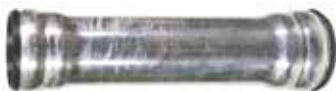
LORO-X Pipe with two sockets, DN 100, the cut pipes can be used as two pipes with one socket Art.-No. 00120.1000 Weight: 5,1 kg
