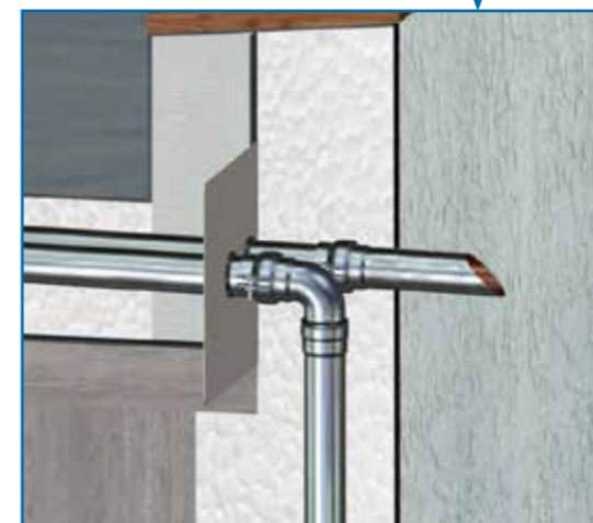
For the penetration through the vapor barrier of pipes that are lying next to each other
