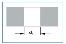
1. Create recess (tapping hole) in concrete ceiling. DN 70:  $d_1 = 132 \text{ mm}$ DN 100:  $d_1 = 162 \text{ mm}$ DN 125:  $d_1 = 192 \text{ mm}$ DN 150:  $d_1 = 252 \text{ mm}$
