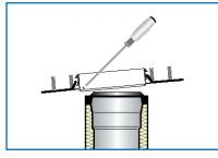
4. Put the first sliding flange onto the LOROFLEX flat roof penetration in a slightly tilted position. Slide on the lower lips of the sealing element with a circular motion of the screw driver and bring the sliding flange into its installation position.
