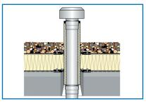
If the room below is ventilated, additionally put on a rain cover. Remove the LORO formwork dome. Result: A clean connection - no rework necessary.
