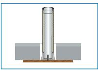
Fasten LORO formwork dome DN 70 or DN 100 on the formwork and insert it into the recess. Create the formwork dome DN 125 and DN 150 on site.
