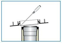
Put the second sliding flange onto the LOROFLEX flat roof penetration in a slightly tilted position.
