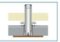
Slide on the first loose flange over the LOROFLEX flat roof penetration, install the vapour barrier and screw together the loose flange and the sliding flange\*. Install the thermal insulation.
