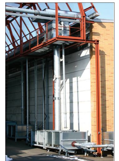
LORO-X test field with up to 100 l/s drainage capacity
