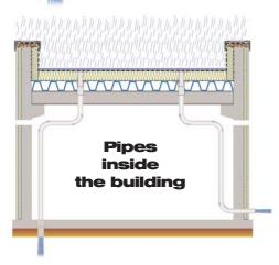
From pitched Roofs with Gutters and downpipe outside the building, it is state of the art to keep the rainwater completely outside the building.
